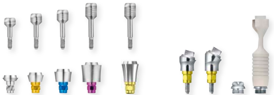
Color-coded MP Abutment Inserts (D 3.4 - 4.5) and MP Insert Screws. The number of grooves on the screw head indicates the gingival height of the matching Abutment Insert.
