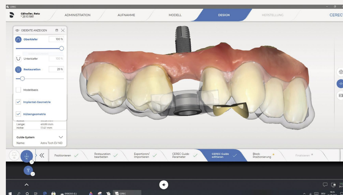
Semi-transparent representation of the CEREC Guide 3 drill template. The metal sleeve is shown, which is glued into the perforation after milling the surgical template.
