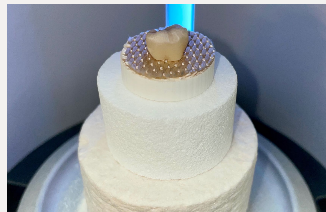
The crown is placed on top of the CEREC SpeedFire honeycomb tray with a firing pad. It must be centered on the pad. The construction is then placed in CEREC SpeedFire.
