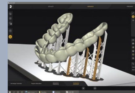
Preparation of print object and fabrication structures
