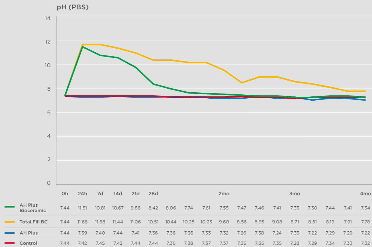
Figure 5: pH of AH Plus Bioceramic Sealer, Total Fill BC Sealer, and AH Plus in distilled water (AD) over 28 days and in PBS over 4 months, respectively.
