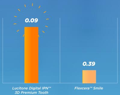
Dentsply Sirona internal 3-Body wear testing at 37 °C, Volume Loss (MM³) @ 400,000 Cycles.
