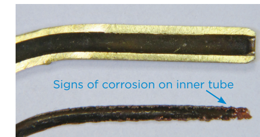
CLOSE-UP OF INNER AND OUTER METAL TUBES
