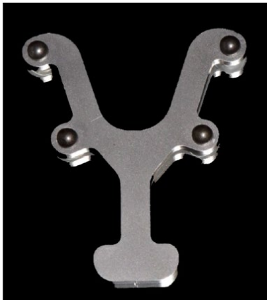
Figure 1. Metallic reference aid with four steel spheres.
