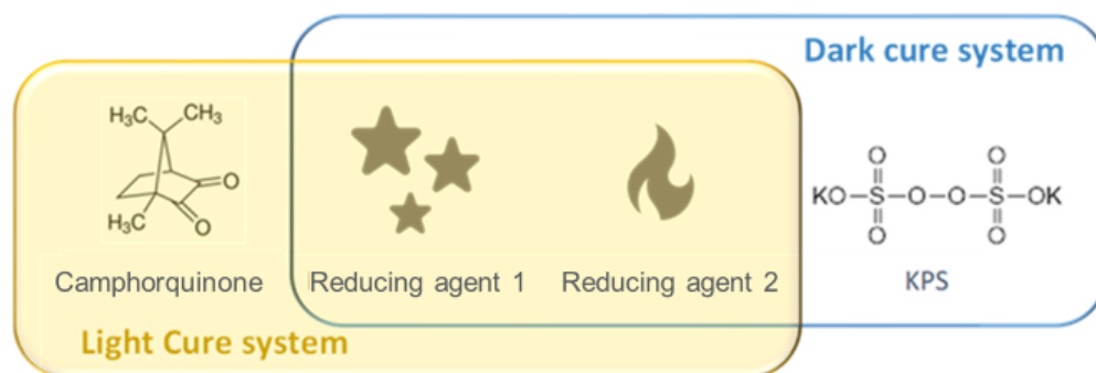
Figure 8 Composition of the unique initiators system of Surefil one
