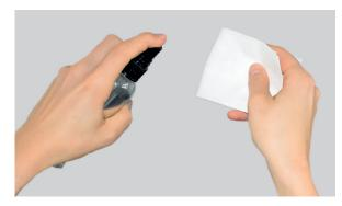
Clean the glass pane with Isopropanol if it is contaminated with resin, with lens cleaner (Purosol) and a microfiber cloth.
