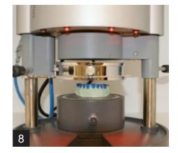
Once the heat time has expired, you will hear a long beep. Pull the lever on the right side (9b), moving the heating element away from the base of the machine. The lever is spring-loaded; be sure to pull past the point of tension and hold while simultaneously pressing the white button on the left side (9a) of the Drufomat Scan. Once the pressure bar on the screen rises to level 2, you can release both the lever and the white button at the same time.
