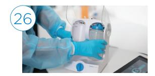
Open shield and remove empty bottle from position "A" and place in position "B".
