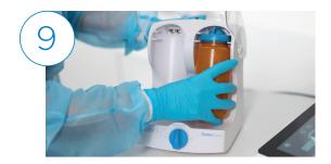
Remove the orange disinfectant bottle from position "A" and place it in position "B" and close the shield.
