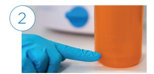
Prepare a 1:10 Sodium Hypochlorite Solution by adding a 5.25% Sodium Hypochlorite to the designated line on the orange disinfectant bottle.
