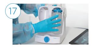
Open the shield. Remove the water bottle from position "A" and place it in position "B".
