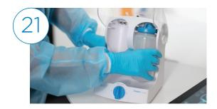
Open the shield and remove the empty bottle from position "B".
