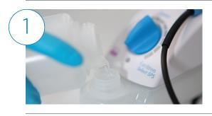
After completing the "Shut-Down Procedures (end of day)" referenced in your Cavitron Select Instructions for Use, begin by preparing a 1:10 Sodium Hypochlorite Solution by mixing 1 part 5.25% Sodium Hypochlorite with 10 parts tap water.
