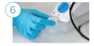
After the minimum 10-minute wait time, unscrew reservoir cap and discard disinfectant solution.
