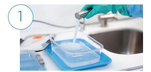
Begin by preparing a pH neutral enzymatic instrument cleaning solution, following the manufacturer's concentration rates.
