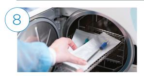
Allow the dry cycle to finish before removing the Cavitron® inserts from the sterilizer.
