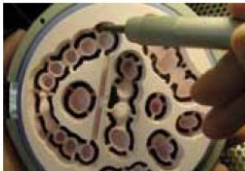
Figure 4: Sandblasting the workpieces.
