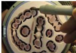
Figure 4: Sandblasting the workpieces.
