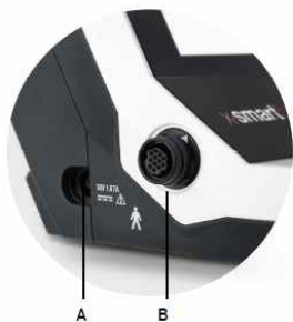
Fig. 4 Power and Motor handpiece connectors
